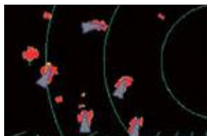
LightHouse II AIS Targets overlaid on radar screen
